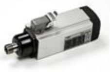
MT1055 - Y6162Y0003 Kw 1-S1/1,30-S6 - connection ER20 collet - 18.000rpm - rated voltage 380V - right rotation
