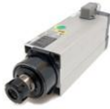
MT1073 - Y6162Y0015 Kw 2-S1/2,40-S6 - connection ER25 collet - 12.000rpm - rated voltage 220V - right rotation
