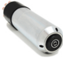
ES327 - H6161H1278 Kw 3,0-S1/3,6-S6 - HSK E25 - 40.000rpm - liquid cooling 380V - special pressurization
