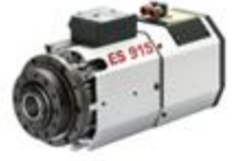
ES915 - H6161H0633 Kw 3,8-S1/4,6-S6 - ISO30 - short nose - 24.000rpm - forced air cooling 220/380V
