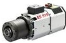
ES915 - H6161H0763 Kw 3,8-S1/4,6-S6 - ISO30 - long nose - 24.000rpm - forced air cooling 220/380V
