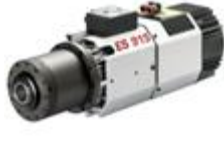
ES915 - H6161H0464 Kw 3,8-S1/4,6-S6 - ISO30 - long nose - 24.000rpm - electric fan cooling 220/380V
