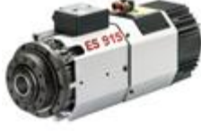
ES915 - H6161H0380 Kw 5,0-S1/6,0-S6 - ISO30 - short nose - 24.000rpm - electric fan cooling 380V
