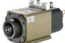
ES326 - H6161H0460 Kw 4,0-S1/4,8-S6 - HSK E25 - 40.000rpm - liquid cooling 380V
