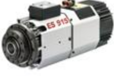
ES915 - H6161H0461 Kw 3,8-S1/4,6-S6 - ISO30 - short nose - 24.000rpm - electric fan cooling 220/380V
