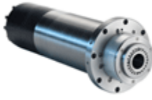
ES334 - H6161H1379 Kw 3,6-S1/4,3-S6 - BT30 - 30.000rpm - liquid 220V - encoder LB 1Vpp
