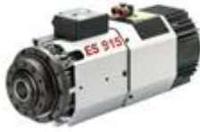
ES915 - H6161H0309 Kw 3,8-S1/4,6-S6 - ISO30 - short nose - 24.000rpm - electric fan cooling 220/380V
