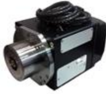
ES793 - H6161H1284 Kw 15,0-S1/18,0-S6 - HSK A63 - 18.000rpm - liquid cooling 380V - opt. rotary joint - encoder LB 1Vpp
