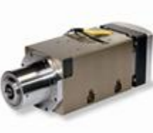
ES789 - H6161H0668A Kw 15,0-S1/18,0-S6 - HSK F63 - long nose - 24.000rpm - liquid cooling 380V
