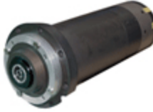
ES332 - H6161H1432 Kw 13-S1/15,6-S6 - HSK E40 - 24.000rpm - liquid cooling 380V - encoder LB 1Vpp - no rotary joint
