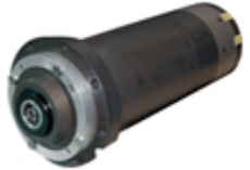
ES332 - H6161H1433 Kw 13-S1/15,6-S6 - HSK E40 - 32.000rpm - liquid cooling 380V - encoder LB 1Vpp - no rotary joint
