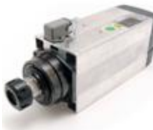
MT1090 - Y6162Y0027 Kw 5,00-S1/6,00-S6 - connection ER32 collet - 12.000rpm - rated voltage 380V - right rotation
