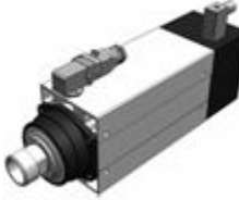
MT1090 - Y6162Y0076 Kw 3,90-S1/5,10-S6 - connection ER32 collet - 18.000rpm - rated voltage 380V - right rotation
