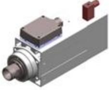
MT1090 - Y6162Y0063 Kw 3,90-S1/5,10-S6 - connection ER32 collet - 18.000rpm - rated voltage 220V - right rotation
