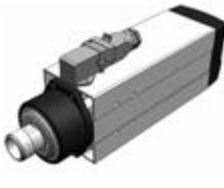
MT1073 - Y6162Y0071 Kw 3-S1/3,60-S6 - connection ER25 collet - 18.000rpm - rated voltage 380V - right rotation
