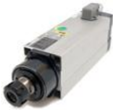
MT1073 - Y6162Y0017 Kw 3-S1/3,60-S6 - connection ER25 collet - 18.000rpm - rated voltage 220V - right rotation
