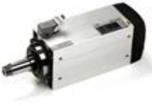
AT1090 - Y6164Y0022 Kw 5,00-S1/6,00-S6 - connection Keyed - 12.000rpm - rated voltage 380V - right rotation
