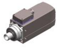
MT1090 - Y6162Y0022 Kw 4,50-S1/5,40-S6 - connection ER32 collet - 18.000rpm - rated voltage 220V - right rotation
