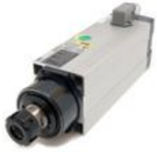
MT1073 - Y6162Y0014 Kw 3-S1/3,60-S6 - connection ER25 collet - 18.000rpm - rated voltage 380V - right rotation
