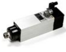
MT1073 - Y6162Y0057 Kw 2,10-S1/2,80-S6 - connection ER25 collet - 18.000rpm - rated voltage 380V - right rotation
