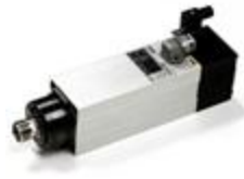
MT1073 - Y6162Y0040 Kw 2,10-S1/2,80-S6 - connection ER25 collet - 18.000rpm - rated voltage 220V - right rotation
