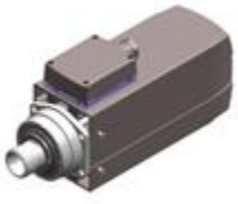
MT1090 - Y6162Y0023 Kw 4,50-S1/5,40-S6 - connection ER32 collet - 18.000rpm - rated voltage 220V - right rotation
