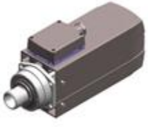
MT1090 - Y6162Y0030 Kw 5,00-S1/6,00-S6 - connection ER32 collet - 12.000rpm - rated voltage 220V - right rotation
