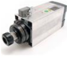
MT1090 - Y6162Y0020 Kw 4,50-S1/5,40-S6 - connection ER32 collet - 18.000rpm - rated voltage 380V - right rotation
