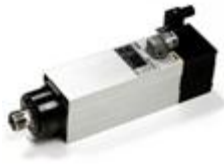
MT1073 - Y6162Y0058 Kw 2,10-S1/2,80-S6 - connection ER25 collet - 18.000rpm - rated voltage 220V - right rotation
