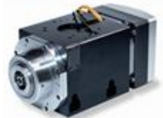
ES779 - H6161H0517A Kw 10,0-S1/12,0-S6 - HSK F63 - short nose - 24.000rpm - liquid cooling 380V - encoder LB 1Vpp - holes
