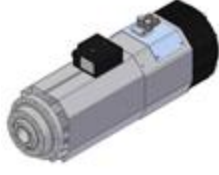
ES929 - H6161H0819 Kw 7,5-S1/9,0-S6 - ISO 30 - short nose - 24.000rpm - electric fan cooling 380V - ceramic bearings
