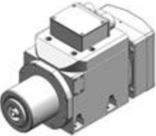
ES779 - H6161H0746 Kw 10,0-S1/12,0-S6 - HSK F63 - long nose - 25.000rpm - liquid cooling 380V - holes - military elect. conn.
