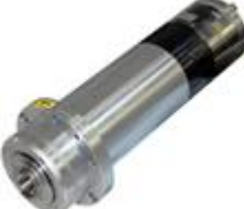
ES331 - H6161H0755 Kw 7-S1/8,4-S6 - BT30 - 24.000rpm - liquid cooling 380V
