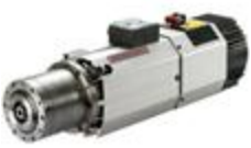
ES929 - H6161H0806 Kw 7,5-S1/9,0-S6 - HSK F63 - long nose - 24.000rpm - electric fan cooling 380V
