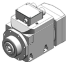
ES779 - H6161H1121 Kw 10,0-S1/12,0-S6 - HSK F63 - short nose - 24.000rpm - liquid cooling 380V - holes - military elect. conn.
