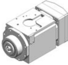
ES779 - H6161H0688 10,0-S1/12,0-S6 Kw - HSK F63 - short nose - 24.000rpm - liquid cooling 380V - encoder LB 1Vpp - special holes
