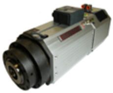
ES929 - H6161H1030 Kw 7,5-S1/8,6-S6 - HSK F63 - short nose - 24.000rpm - forced air cooling 380V
