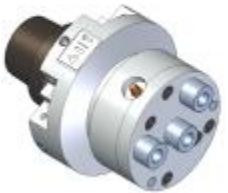
code HASP0140 (HSK E63) 3 vertical outlets 52-16mm for hinges
