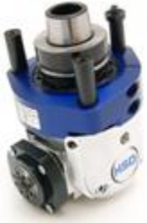
code H6314H0304 (HSK F63) Available with HOMAG coupling 1 blade outlet + ER25 collet. For inclined cutting/milling
